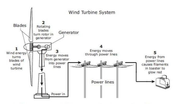
In the diagram above, a wind turbine is transforming energy from the wind. Between which two steps in the diagram is mechanical energy being converted into electrical energy?
